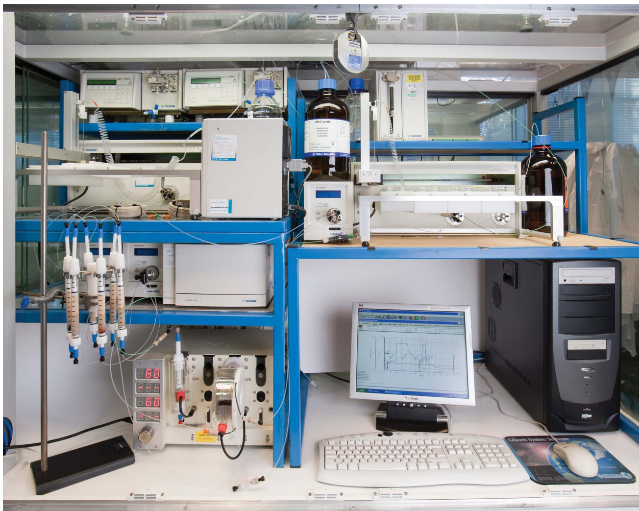
Fig. 7 Automated reactor for the flow synthesis of 5-amino-4-cyano-1,2,3-triazoles as depicted in Scheme 4.
